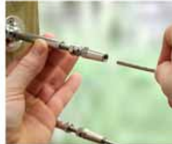
Step 1 Fully seat wire rope.
